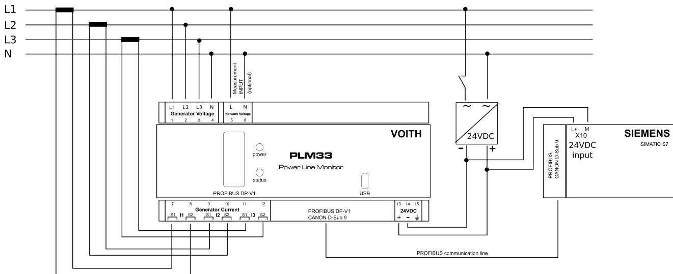
PLM33 allows measurement in TN, TT and IT networks. In case of IT network measurement N (4) pole is not connected.
